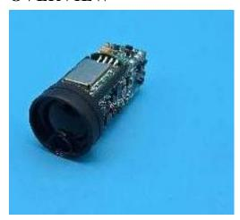
LRF1200A1 laser ranging module is a new lightweight and compact ranging module, operating at a wavelength of 905nm. The maximum range of the product is ≥1200m, using a UART-TTL interface and supporting test software, which is convenient for users to further develop. It has the characteristics of small size, light weight and reliable performance. It can be used in aviation, communications, geology, police, outdoor sports and other occasions.
