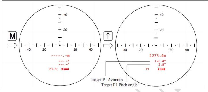
Aim for the second target,press "↑" to complete measurement target P2. Press "↑" again to complete measurement distance between P1 and P2.
