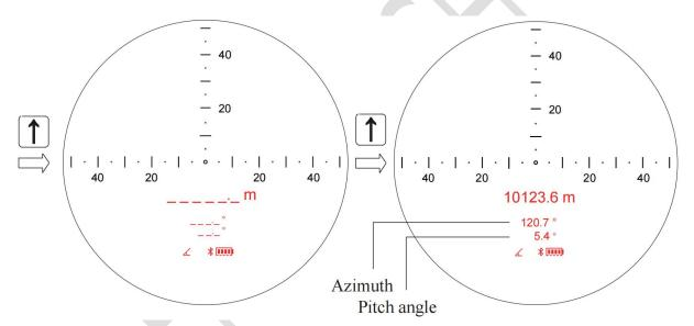
Long press "↑" to continuous ranging at ranging and angle mode,release to stop. \* Angles are not displayed when continuous ranging or measuring multiple targets. Up to measuring 3 targets in multi-target.
